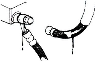
( leak, damaged, looseness of brake line )
